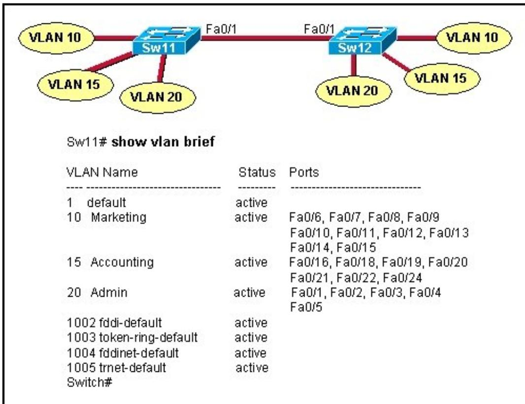
A technician is troubleshooting host connectivity issues on the switches. The hosts in VLANs 10 and 15 on Sw11 are unable to communicate with hosts in the same VLANs on Sw12. Hosts in the Admin VLAN are able to communicate. The port-to-VLAN assignments are identical on the two switches. What could be the problem?
