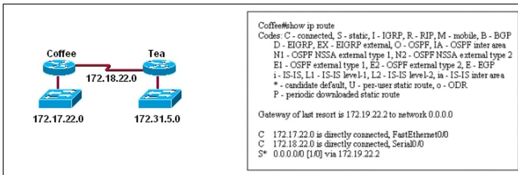
Based on the output of the show ip route command and the topology shown in the graphic, what is the cause of the failure?
