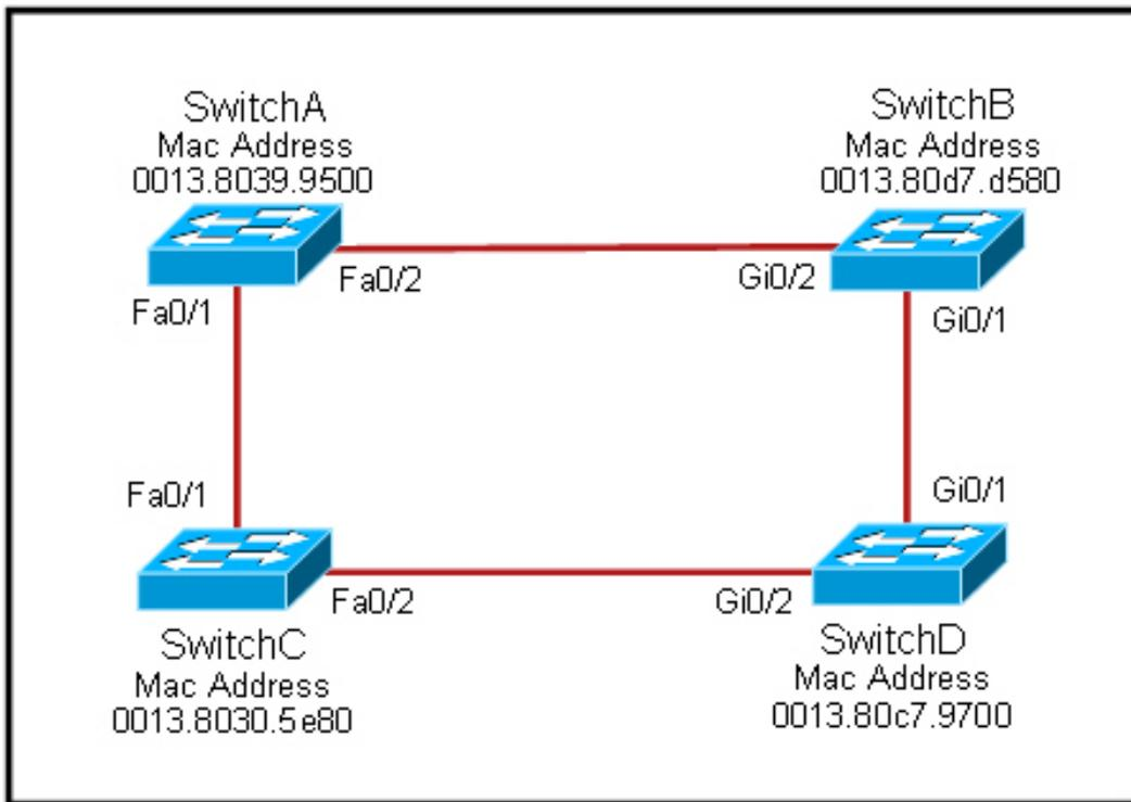
Each of these four switches has been configured with a hostname, as well as being configured to run RSTP. No other configuration changes have been made. Which three of these show the correct RSTP port roles for the indicated switches and interfaces? (Choose three.)
