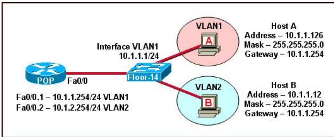
The network shown in the diagram is experiencing connectivity problems. Which of the following will correct the problems? (Choose two.)
