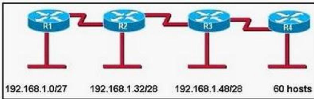
A new subnet with 60 hosts has been added to the network. Which subnet address should this network use to provide enough usable addresses while wasting the fewest addresses?
