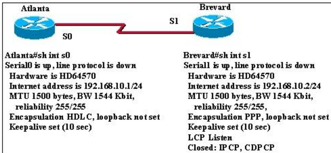
Given the partial configurations, identify the fault on the Brevard router that is causing the lack of connectivity.
