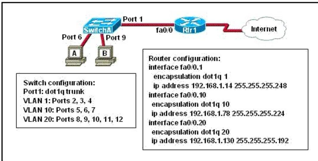
A network administrator is adding two new hosts to SwitchA. Which three values could be used for the configuration of these hosts? (Choose three.)
