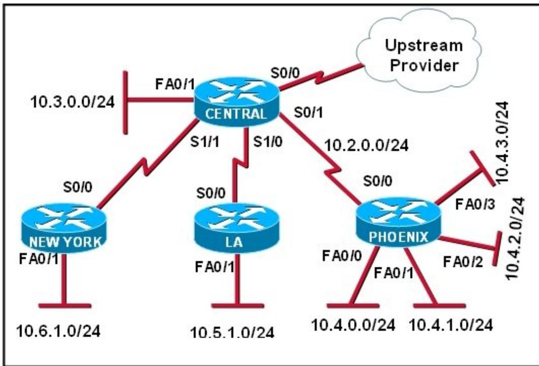
The Lakeside Company has the internetwork in the exhibit. The administrator would like to reduce the size of the routing table on the Central router. Which partial routing table entry in the Central router represents a route summary that represents the LANs in Phoenix but no additional subnets?
