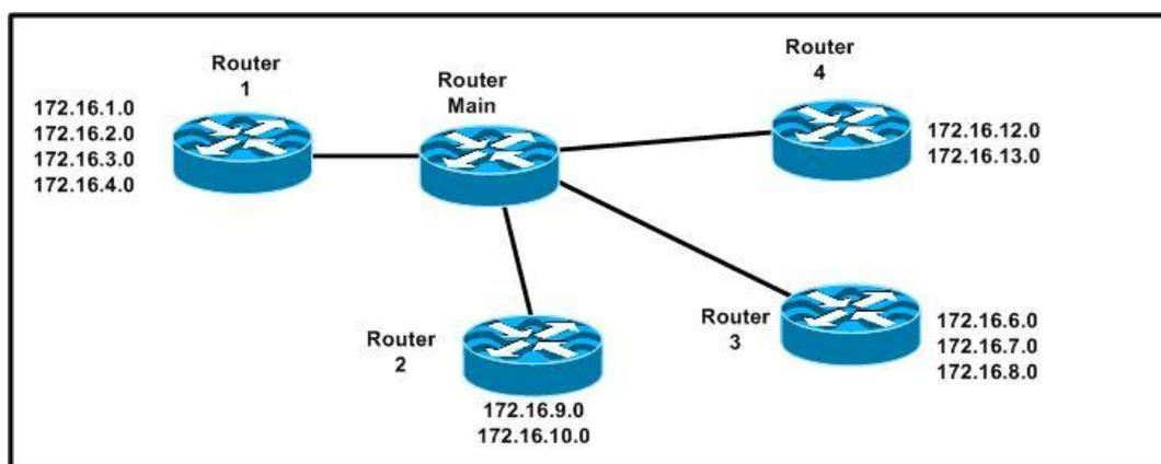
Which address range efficiently summarizes the routing table of the addresses for router Main?
