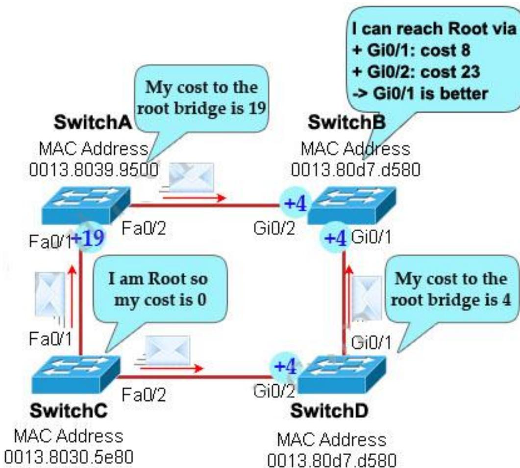
SwitchC advertises its cost to the root bridge with a value of 0. Switch D adds 4 (the cost
