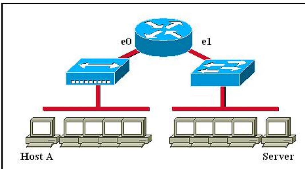
Host A is communicating with the server. What will be the source MAC address of the frames received by Host A from the server?
