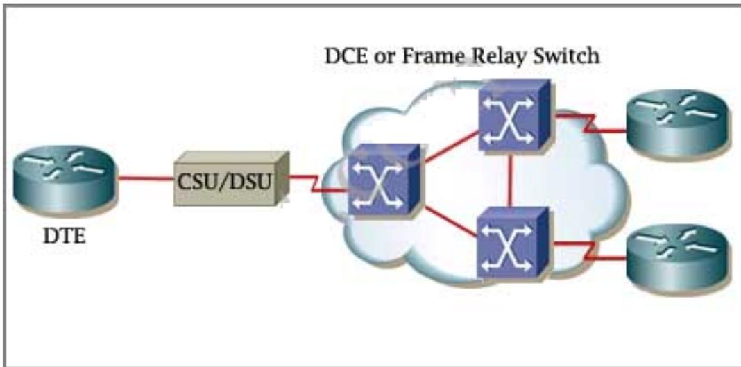
A modem modulates outgoing digital signals from a computer or other digital device to analog signals for a conventional copper twisted pair telephone line and demodulates the incoming analog signal and converts it to a digital signal for the digital device. A CSU/DSU is used between two digital lines -
