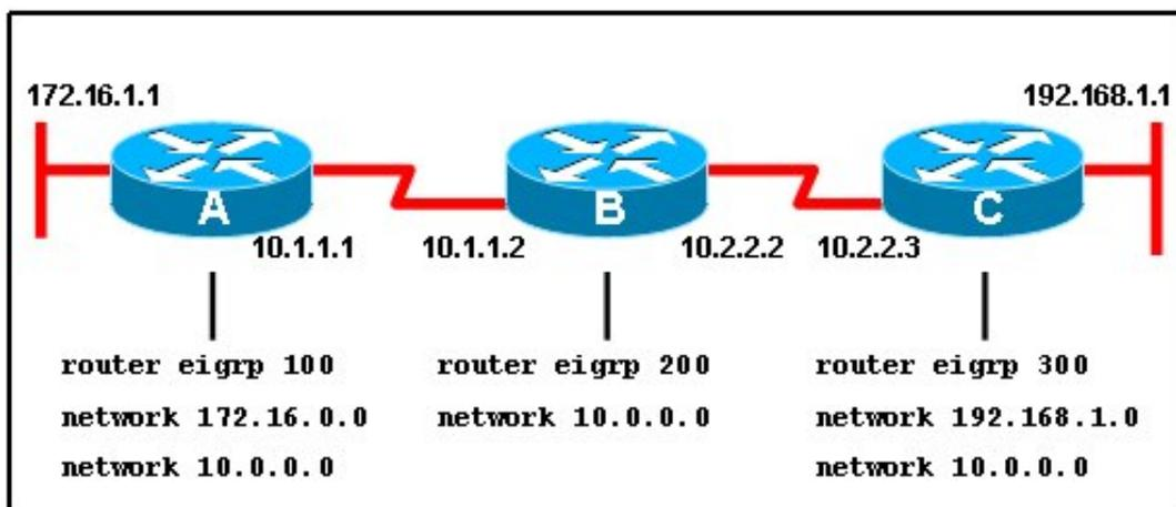
When running EIGRP, what is required for RouterA to exchange routing updates with RouterC?
