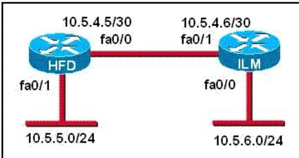
A static route to the 10.5.6.0/24 network is to be configured on the HFD router. Which commands will accomplish this? (Choose two.)
