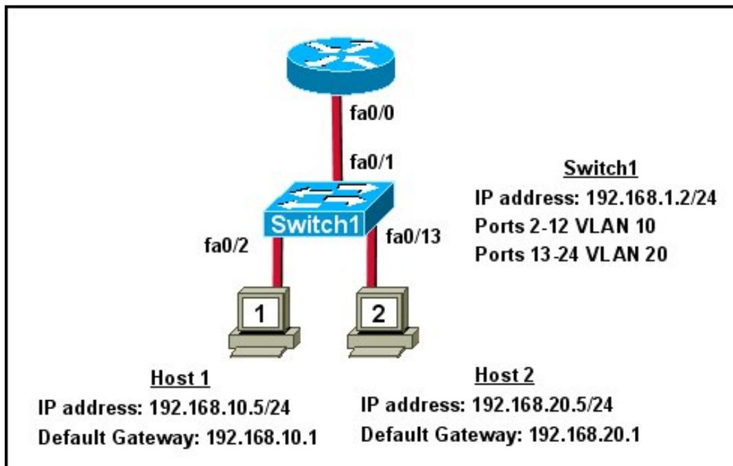
What commands must be configured on the 2950 switch and the router to allow communication between host 1 and host 2? (Choose two.)
