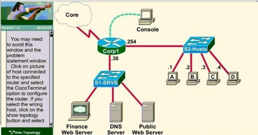
Access to the router CLI can be gained by clicking on the appropriate host.
