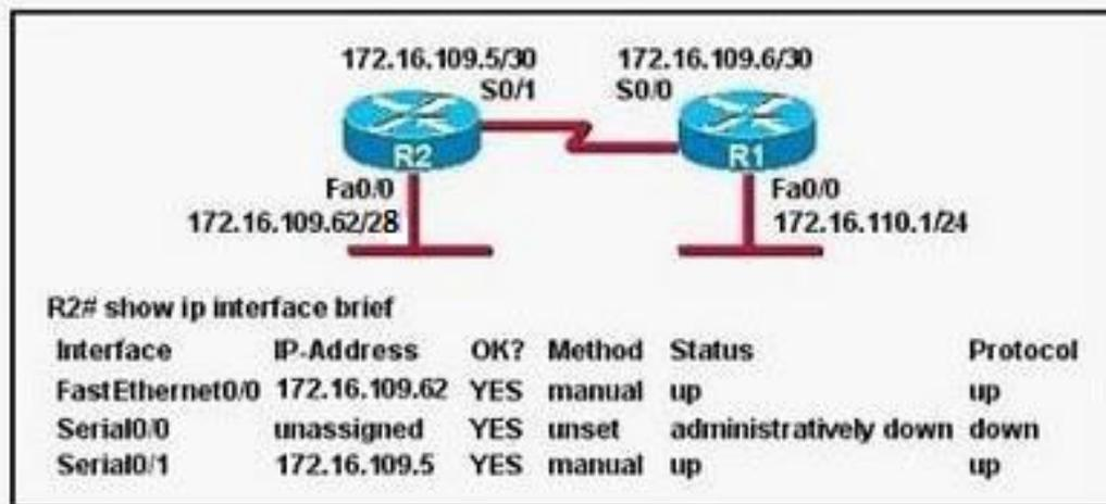
Assuming that the entire network topology is shown, what is the operational status of the interfaces of R2 as indicated by the command output shown?
