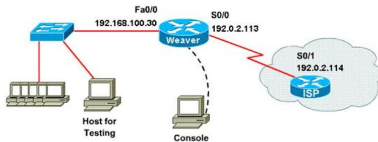
A network associate is configuring a router for the weaver company to provide internet access. The ISP has provided the company six public IP addresses of 198.18.184.105 198.18.184.110. The company has 14 hosts that need to access the internet simultaneously. The hosts in the company LAN have been assigned private space addresses in the range of 192.168.100.17 – 192.168.100.30.
