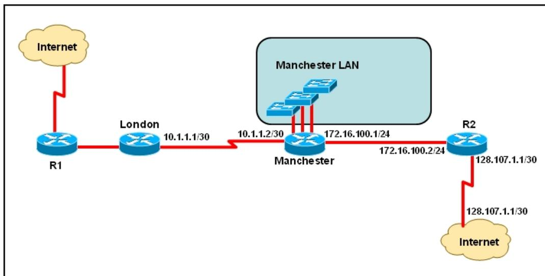
The speed of all serial links is E1 and the speed of all Ethernet links is 100 Mb/s. A static route will be established on the Manchester router to direct traffic toward the Internet over the most direct path available. What configuration on the Manchester router will establish a route toward the Internet for traffic that originates from workstations on the Manchester LAN?
