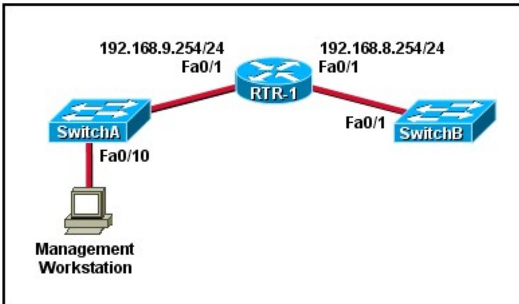
A technician has installed SwitchB and needs to configure it for remote access from the management workstation connected to SwitchA. Which set of commands is required to accomplish this task?
