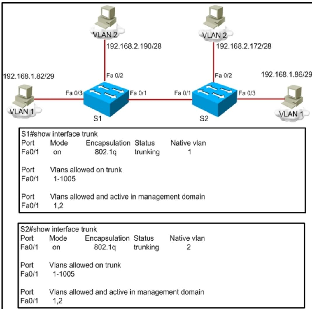
A frame on VLAN 1 on switch S1 is sent to switch S2 where the frame is received on VLAN 2. What causes this behavior?
